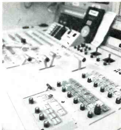
GVG 1600-3F switcher in production area of Bay Area Mobiletape truck.
