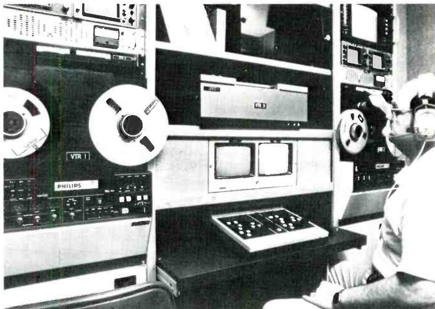
Videotape operator Al Campbell performs insert edit with Philips recorders in taping facility of van.
