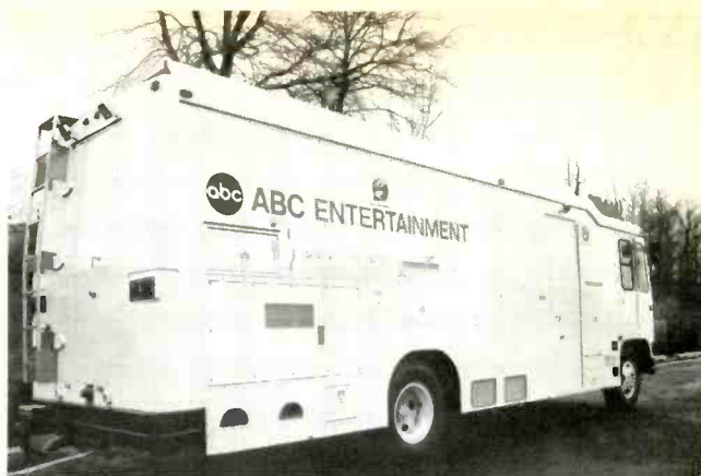
ABC's "mini-mobile" unit is a three-camera entertainment-type truck, a good example of the medium-sized straight truck.
